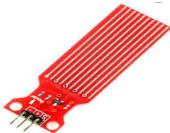
Fig-8: Water Level Sensor
