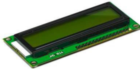
Fig-11: Liquid Crystal Display
