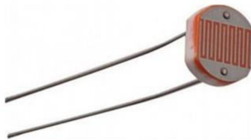
Fig-7: Light Dependent Resistor
